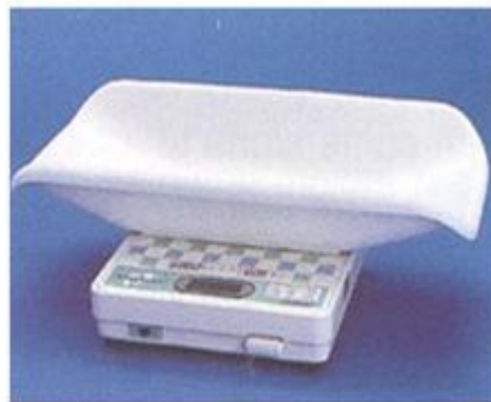
Photo 4-66: Weighing a baby with this type of scale can accurately weigh up to a few ounces. [Source: Medela]
